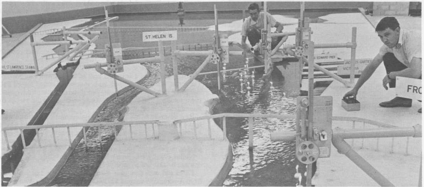
View of hydraulic model showing luminous floats used on model to determine current velocities in the area of Ile Ste-Helene. The technician, shown at right, records current velocity with the help of a chronometer.
