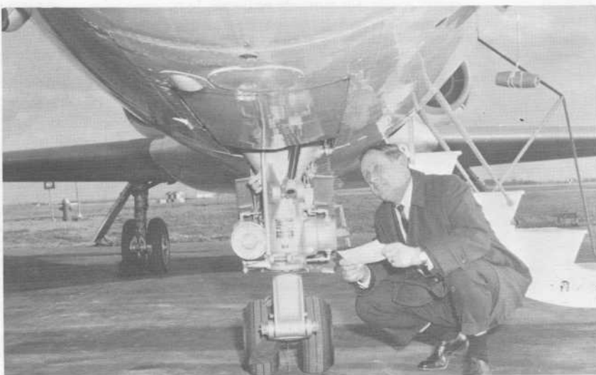
Airworthiness Inspector T. A. Parry checks nose landing gear on FanJet Falcon after its importation by Imperial Oil Company.
