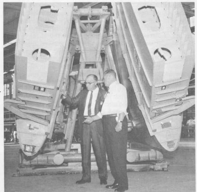
Above and below, Airworthiness Inspector W. L. Brown and Douglas Superintendent Inspector M. Boyd (in shirtsleeves) examine a completed DC-9 wing prior to shipping from Toronto to Douglas Aircraft, Long Beach, California for assembly of the complete aircraft.
