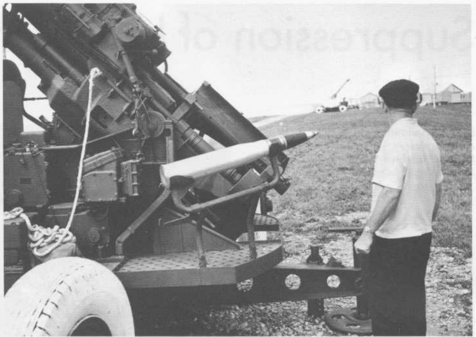
A 100 millimeter gun and silver iodide shell used for hail suppression in the U.S.S.R.
