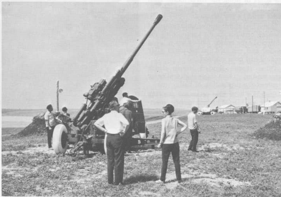
A 100 millimeter gun used for firing silver iodide shells into hail clouds.
