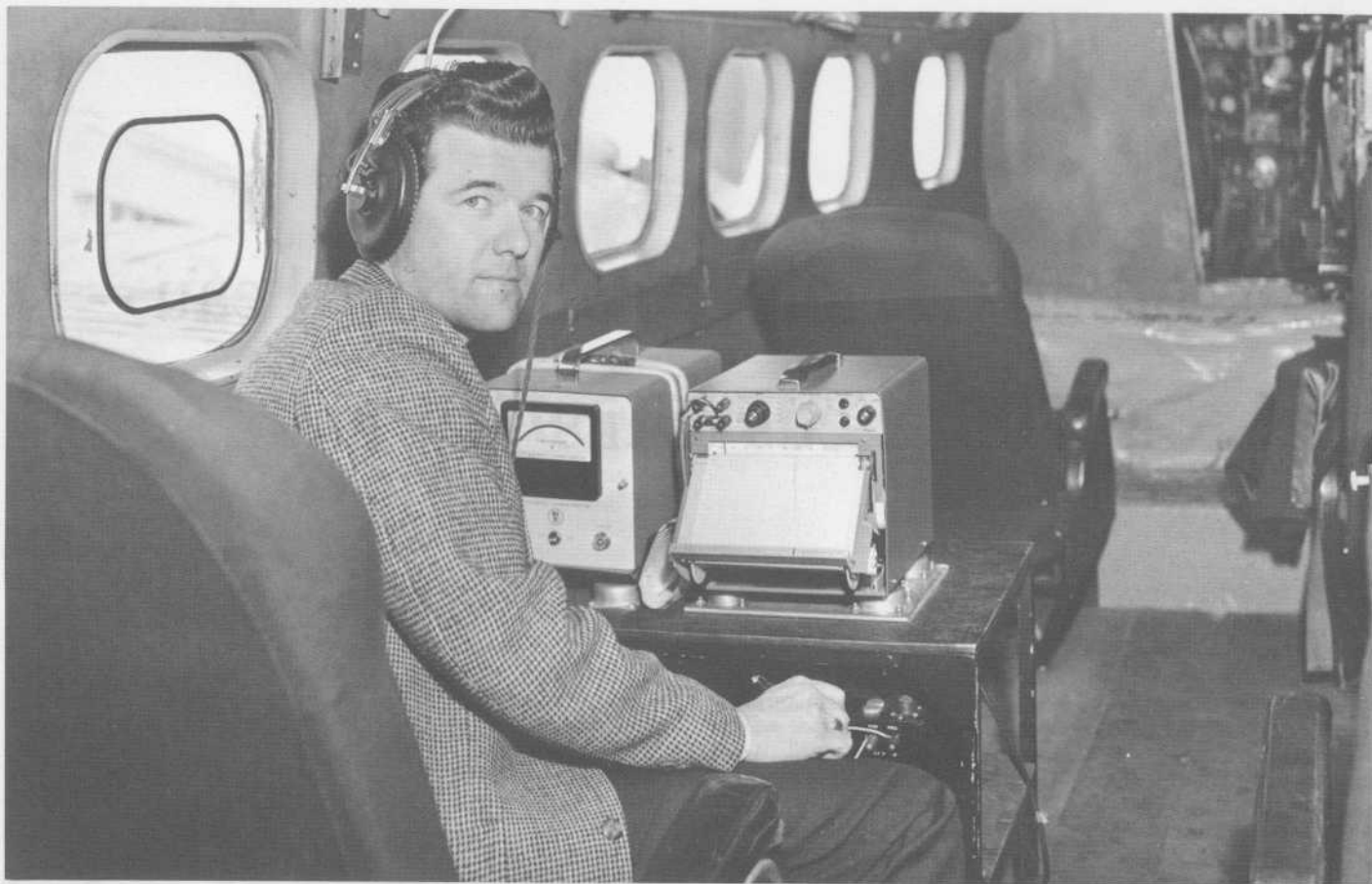
Research Assistant Don Massey sits at the controls of the airborne radiation thermometer through which he records lake temperature while in flight.
