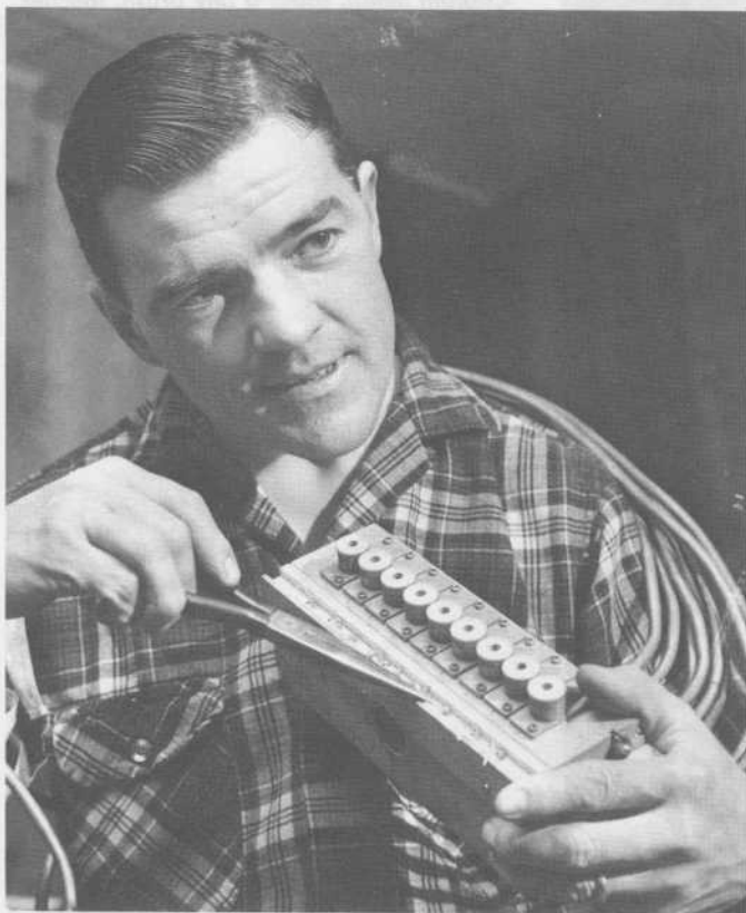
Ted Devey examines the organ's magnet box—an electro-pneumatic component.
