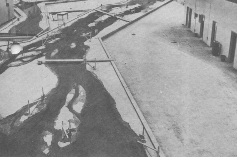
◀ Bird's eye view of Transport Department's giant working model of St. Lawrence ship channel at Ville LaSalle, Que. Looking downstream, large island in left foreground is Ile Ste.-Therese. Long island in centre is Ile de Vercheres. Upper section of model represents stretch from Bout de l'Ile (to left of Ile Ste. Therese, where Ottawa river joins St. Lawrence) to Lanoraie near rear wall. Lower section of model, seen left of upper section, represents stretch downstream from Lanoraie to Lake St. Peter, with Sorel Islands in centre background. Gallows-like instruments throughout model are gauges recording water levels.
