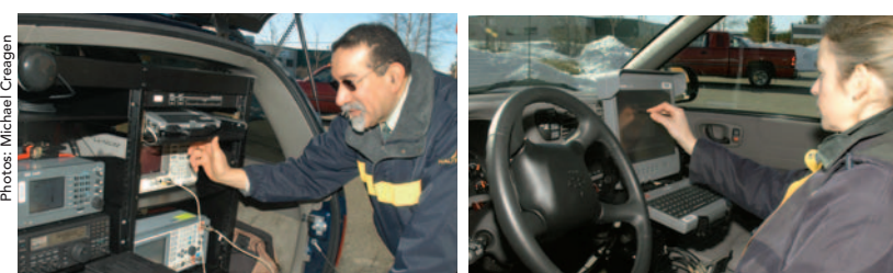
Photos: Michael Creagen. Spectrum Management Officer Manuel Escobar shows the electronic equipment in the rear of the branch’s mobile monitoring vehicle, which is in turn remotely controlled by computer by Management Officer Gwen Arthurs from the operators position in the front of the vehicle.
